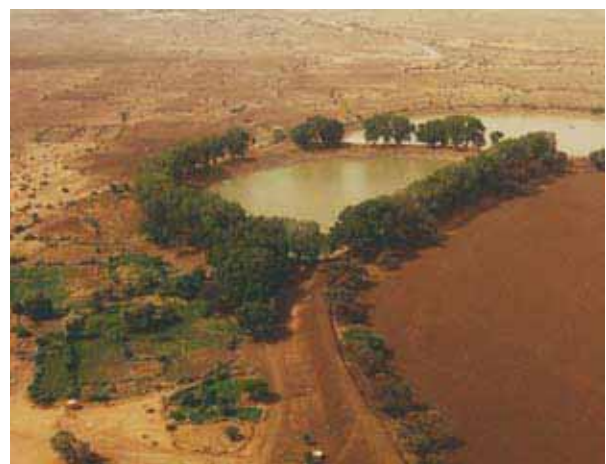
A small dam complex in Darfur, with a banked catchment area, storage dams and associated small-scale irrigated agriculture
