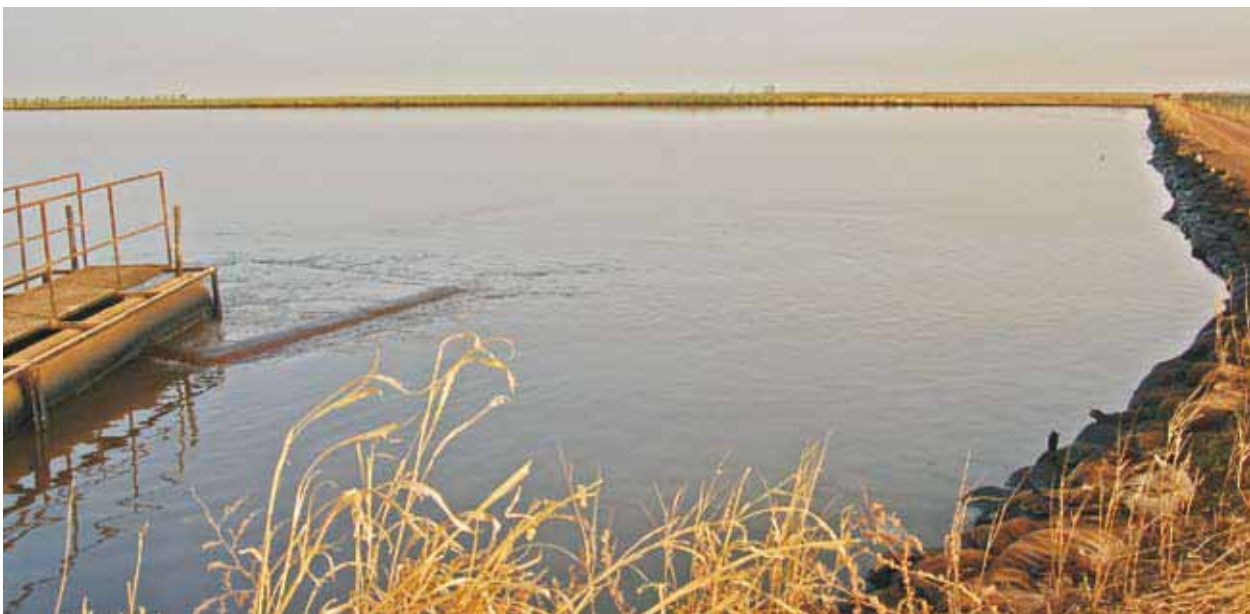
Produced water flowing into a holding pond at Heglig. Produced water can be difficult and expensive to treat, but has serious impacts on the environment if released untreated
