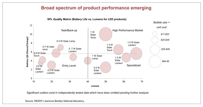
Figure 4: Solar Portable Light Performance Matrix
