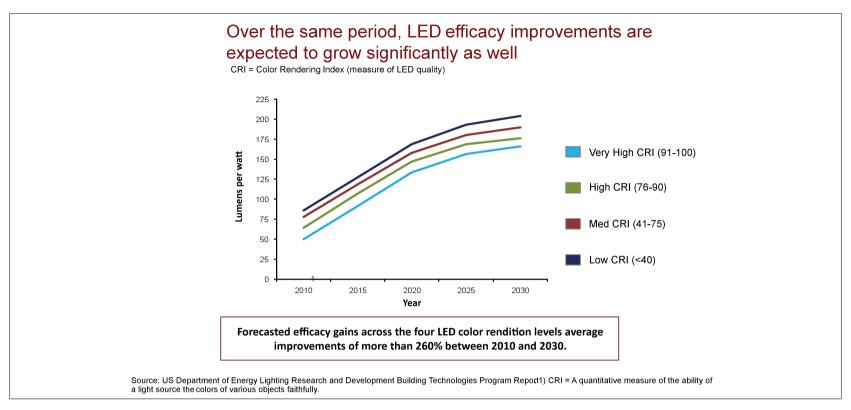
Figure 18: Forecast on LED efficiency
