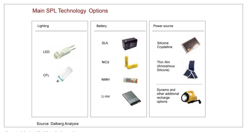
Figure 3: Solar Portable Light technology options
