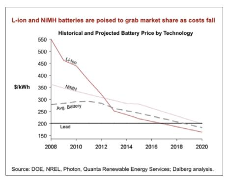
A number of factors may hold back Li-lon adoption in SPL devices, including the need for more expensive electronics (e.g., charge controllers) to ensure safety, charge indicators to avoid over or undercharging, and most significantly, the current lack of easily available Li-lon battery replacements in African markets. Nonetheless, the mobile market saw Li-lon batteries take substantial share from NiMH while facing many of the same issues.
