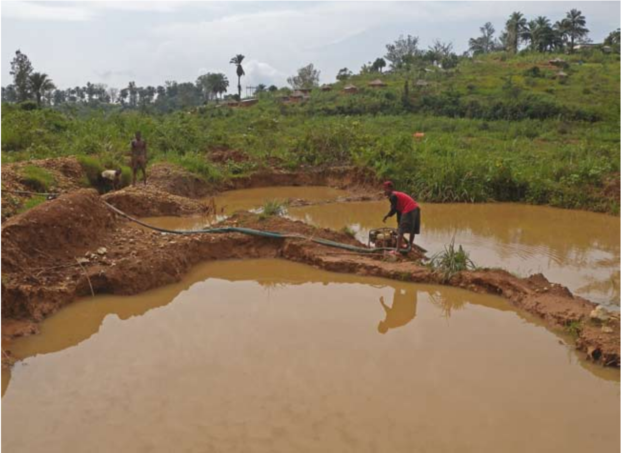
Water-pumps used by artisanal gold miners to wash down the soil releases large amounts of sediment-laden runoff into watercourses and lakes. Mongbwalu, Ituri District
