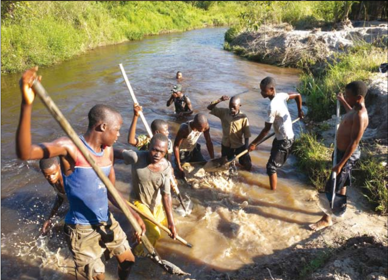
Along the Chibungu River in Kasai Occidental, alluvial diamond mining involves vegetation and soil removal and subsequent washing of the gravel, resulting in increased river turbidity and siltation
