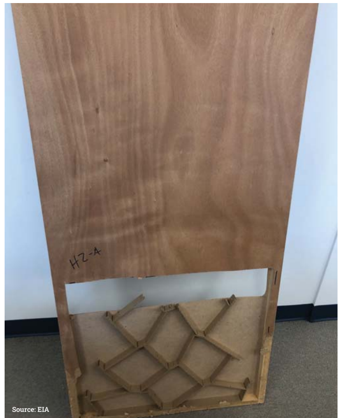
Figure 3 Structure of the Jeld-Wen door
