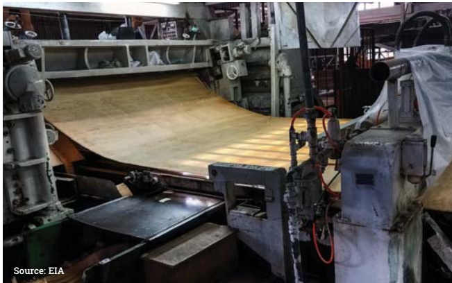
Figure 5 Peeling of okoume log in China
